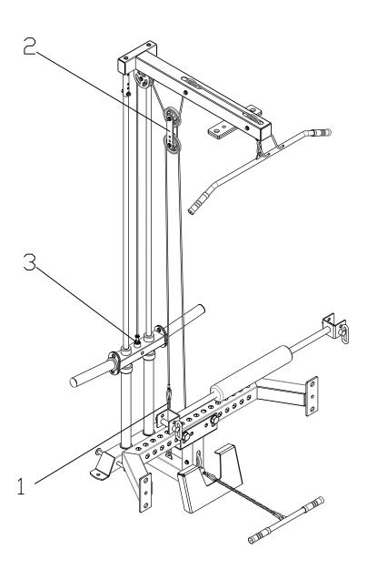
\*The cable tension can be controlled by adjusting 1. Iron chain 2. Pulley support plate 3. Fine tuning bolt
